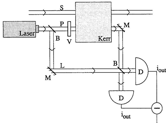
fig. 1 *Kerr QND measurement of photon number. A signal beam S is mixed with a probe beam P into a non-linear medium. The outgoing probe beam is fed into a homodyne detector. [V is a delay, B's are beamsplitters, M's are mirrors, D's are detectors, and L indicates the homodyne local oscillator beam.]*
